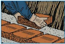
Set the center side alignment groove directly above the backmost 5/8" set back groove of the stones in the next lower layer. See stones at top of this page. Use this visual alignment for each successive layer of stones. Mat material can be used to filter soil fines that may migrate into your clean granular fill. A flexible drain tube is a competent way to assure drainage from behind your wall. As successive layers are set, stagger the face seams of the stones for interlocking wall strength.
